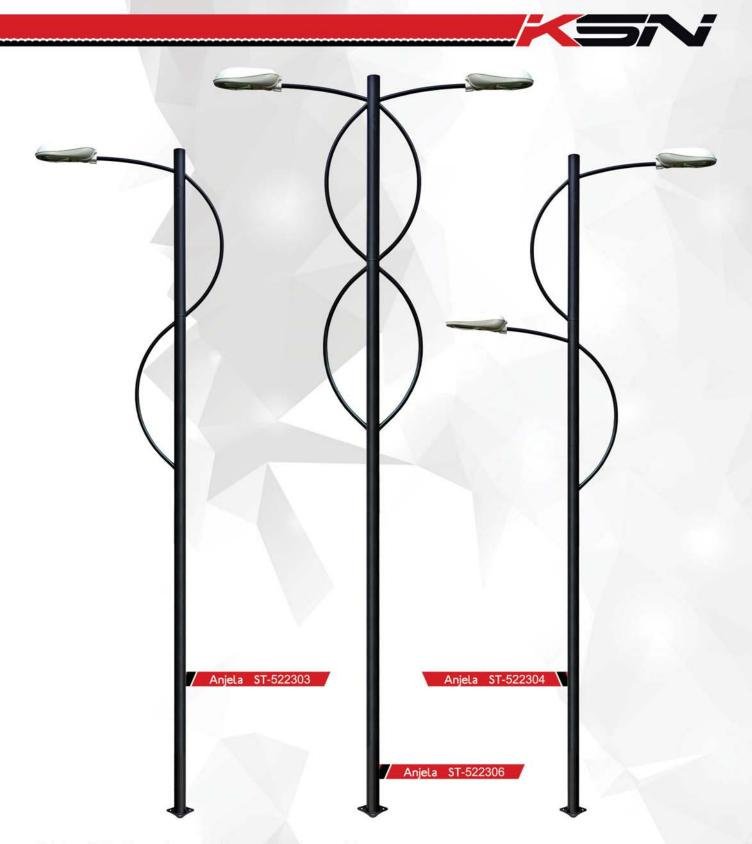
**Anjela:** Light fixture is made die-cast aluminum ,with electrostatic powder coating .Inner reflector is made of anodized aluminum. Tempered glass , resistant against impact and thermal shock and silicon gasket for ingress protection.
