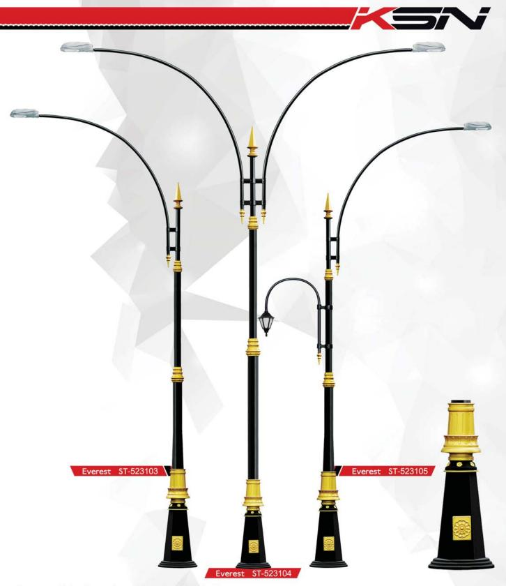
**Everest**: light fixture is made of made of die-cast aluminum, with electrostatic powder coating, and reflector is made of anodized aluminum. tempered glass, resistant against impact and thermal shock, with silicon gasket for ingress protection. pole is made of steel with aluminum cover and celluosic coating resistant against corrosion.
